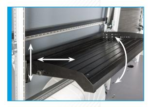
Shelf adjustable towards the vehicle wall, in height and in the inclination angle.
