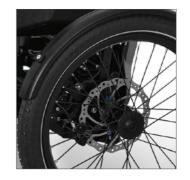
The **hydraulic** Tektro Auriga Twin **disk brake system** won't let you down, even when the bike is fully loaded.
