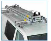
suitable for 1-, 2-, or 3-stage ladders; max. ladder length up to 1.5 times the length of the cross member spacing of the TopSystem; the cross member spacing can be varied from 1380 to 3000 mm up to 35 kg load
