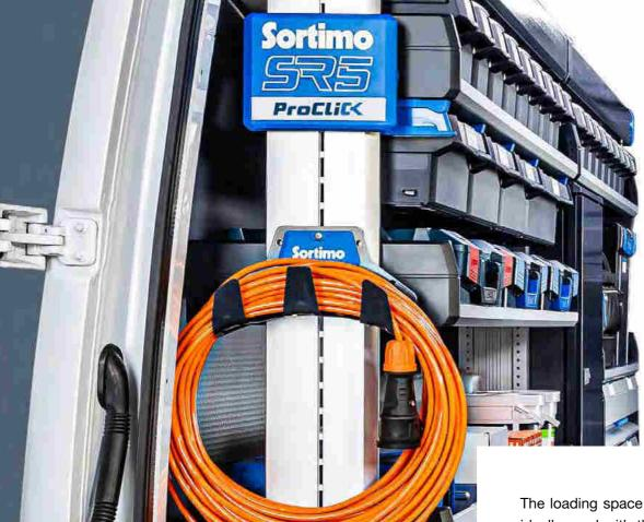
The loading space of the vehicle is ideally used with the SR5 concept. The compact side profiles require considerably less space than the frame construction of conventional van racking systems. In addition, ProClick is copatible with the side profiles so that tool bags or SR5 accessories can be hooked into the ProSafe perforations without using tools. Variation in the component depths and installation position means that the van racking system ideally adapts to the contour of the vehicle.
