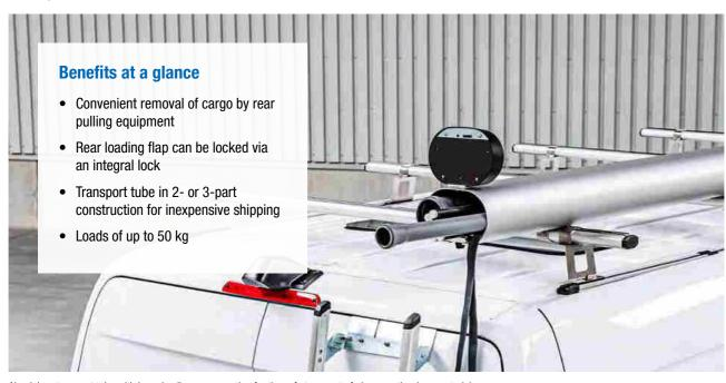
Aluminium transport tube with large loading cross-section for the safe transport of pipes or other long materials.
